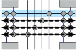
**Figure 1: Channel with four tracks, one of which is reserved. Three nets saturate the three base tracks.**
