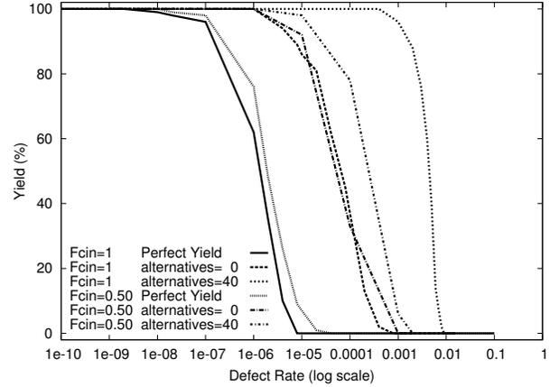
**Figure 3: Yield vs. defect rate for DES with depopulated and fully populated C-Boxes (no extra base tracks, 20% reserved tracks, depopulated case sets  $W_{min}$ )**
