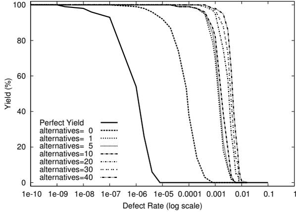
**Figure 2: Yield vs. defect rate for DES with 20% extra base tracks and 20% additional reserved tracks**
