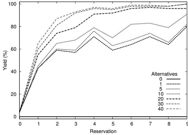
Figure 6: Effects of dividing extra tracks between the base route and alternatives (DES with  $1.4W_{min}$  total tracks, defect rate 0.001)
