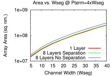
Fig. 6. Area Impact of No Physical Separation
