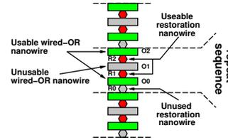
Fig. 4. Restoration Assignment Sequence which Allows us to Restore Two-Thirds of the Wired-OR Terms without Requiring any Physical Isolation
