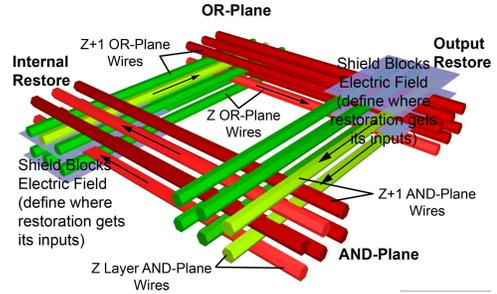
Fig. 3. Redefined Logical Nanowire Layer with Physical Isolation
