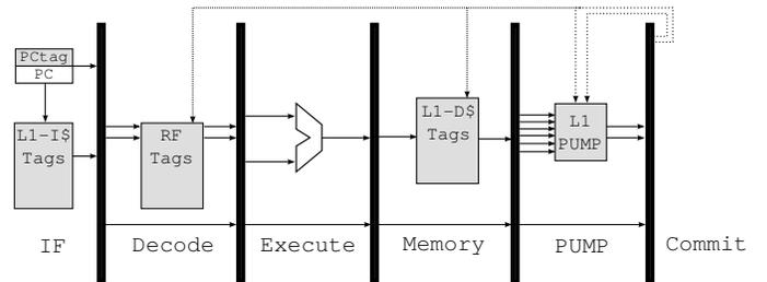
Figure 1: L1 PUMP cache in a processor pipeline
