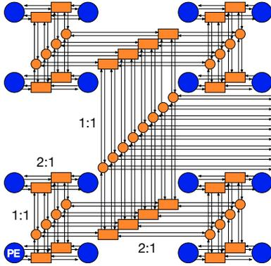
Fig. 2. Spatial Design: HSRA-Style Interconnect with Directional Drive
