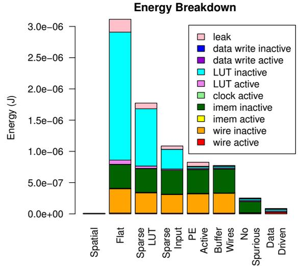
Fig. 6. Impact of Processor and Interconnect Optimizations for stereovision2 for  $S = 8$ ,  $p_t = 0.5$
