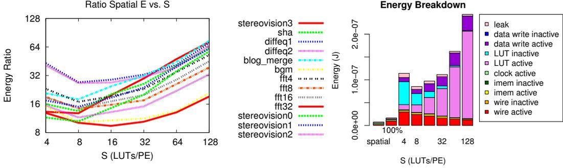
Fig. 9. Impact of PE sequentialization ( $S$ ) on all benchmarks (left) and energy breakdown for *stereovision2* (right) at  $p_t=0.5$
