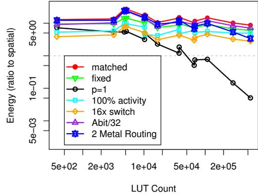
Fig. 12. Net Energy Ratio to Spatial for Data-Driven, Time-Multiplexed  $S = 8$ ,  $p_t = 0.5$  Architecture versus Benchmark LUT Count
