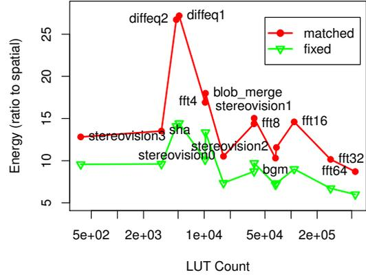
Fig. 11. Net Energy Ratio to Spatial for Data-Driven, Time-Multiplexed  $S = 8$ ,  $p_t = 0.5$  Architecture versus Benchmark LUT Count
