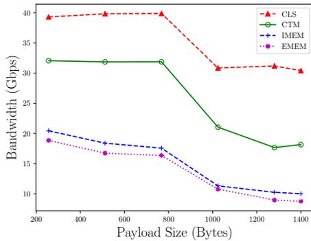
**Figure 8: Intra-packet Regex Matching Performance: DFA location and payload size affect throughput when shared code mode and reduced threads mode are off.**
