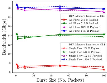
Figure 14: Inter-Packet BW vs. Burst (320 Flows)
