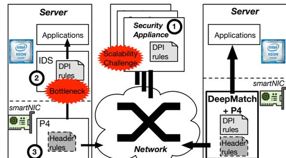
Figure 1: DPI today (left and network) is limited by performance, scalability, and programming/management complexities (shaded red) inherent to the underlying deployment models. DeepMatch (right) pushes DPI into the commodity SmartNICs currently used to accelerate header filtering and integrates DPI with P4, which improves performance and scalability while enabling a simpler deployment model.
