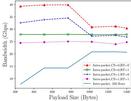
Figure 9: Intra- and Inter-Packet Performance on 320 Flows. CS=shared code mode, RT=reduced thread mode (CS=1 and RT=1 for the Inter-packet case).
